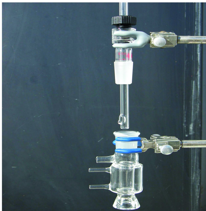
Figure 4. Evaporation chamber with well for liquid chemical reservoir.
